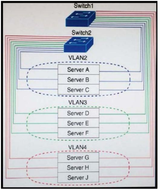
Two Layer 2 Cisco Nexus switches are connected to application servers in a data center. Server A cannot communicate with servers that are in VLANs 3 and 4, but t can communicate with server B and C. What is the cause of the problem?
