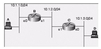
A.This will not work because Router B has no idea of how to forward traffic to the 10.1.3.0/24 network.
