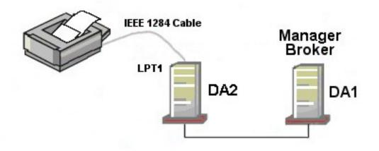
You need to configure a special purpose thermal-transfer printer for your organization. Because it doesn't have a built-in network interface, you've connected it to LPT1 on your DA2 server using a parallel cable. The Printer Agents for your organization's printers are managed by an iPrint Manager and Broker on your DA1 server.
