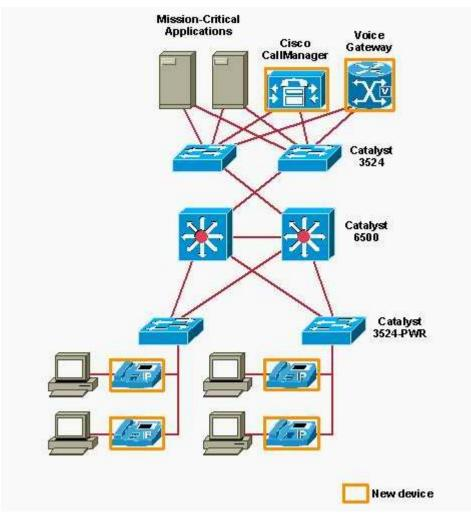
A.The trust boundary should be extended from the 3524-PWR access switches to include the IP phones. B.Ingress rate-limiting should be configured on 3524-PWR access switches to ensure Voice over IP bandwidth guarantees.
