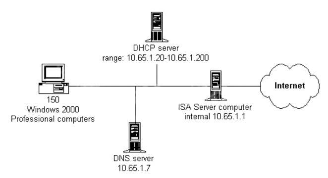
The network uses a root DNS server with the IP address 10.65.1.7 to host the DNS zones for the Windows 2000 domains. The ISA Server computer uses the DNS server of your ISP for name resolution. You want to configure the Web browser on the client computers so that internal and external DNS names are resolved correctly. Company policy specifies that you cannot install the Firewall Client software. Which two actions should you take? (Each correct answer presents part of the solution. Choose two.)
