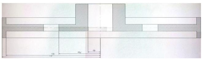
This section view was dimensioned using Baseline Dimensions The dimensions are too close together which impacts the drawing's legibility.
