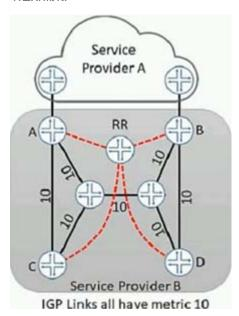
You work for service provider B that wants to implement a hot potato routing policy on the network so that router C uses link C-A to reach service provider A's advertised routes and router D uses link D-B to reach Service Provider A's advertised routes Currently traffic from router C is traversing the core to exit the network on router B.
