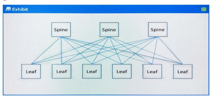
A customer has a 3-stage Clos architecture with three spine devices as shown in the exhibit. If a single spine device fails, what percentage of the remaining bandwidth will be available from leaf node to leaf node?
