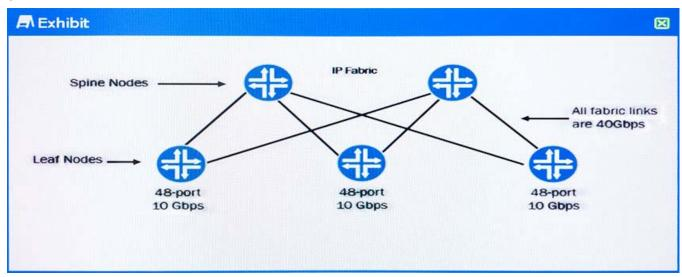
Referring to the exhibit, which hardware change would be made to the IP Fabric to ensure an exact 4:1 oversubscription ratio?
