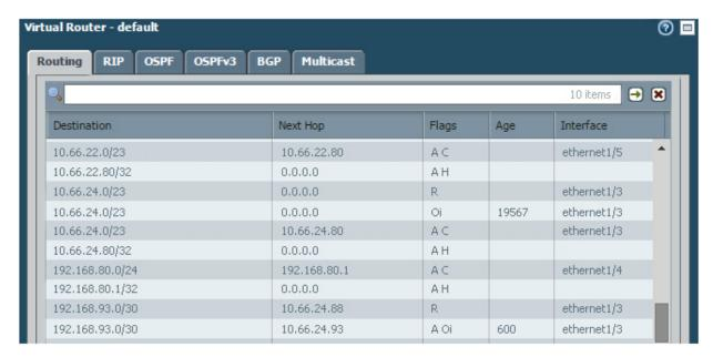
Which configuration change on the firewall would cause it to use 10.66.24.88 as the next hop for the 192.168.93.0/30 network?
